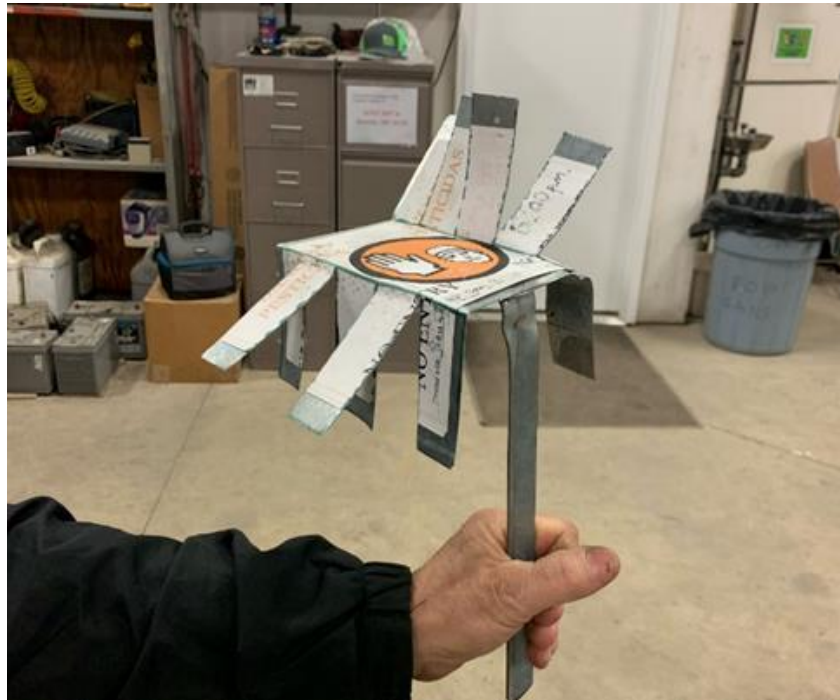
Figure 1. Water sensitive tape was attached to each tab on the contraption to simulate spray coverage on either sugarbeet or waterhemp.
